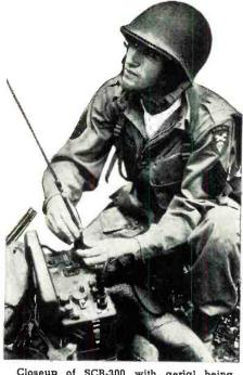
Closeup of SCR-300 with aerial being extended for above-ground operations.
