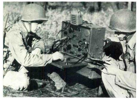
The SCR-284 in operation immediately after glider landing. Photo shows equipment mounted in handcart for rapid maneuverability.
