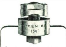
Saves hours of work cutting clean, accurate holes in radio chassis—for connectors and other receptacles. Simply insert cap screw in hole to be enlarged (drill small hole if necessary), turn with ordinary wrench to force punch through the metal. No reaming or filing—hole is smooth and clean. No distortion—die supports metal. Ten sizes from ¾" to 2¼"; also up to 3½" for meters. Write for free catalog 33E to Greenlee Tool Co., 1883 Columbia Ave., Rockford, Ill.
