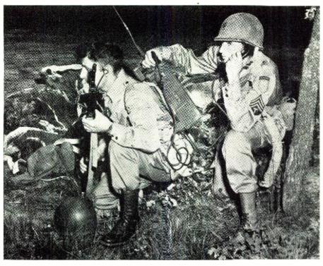
SCR-300 shown in operating position, directly after landing via parachute.
